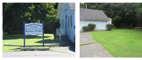
Stormwater currently drains from the property to the surrounding area. Parking spots adjacent to the south building and in the north parking lot can be replaced with porous asphalt to capture and infiltrate roof runoff. Installing rain gardens adjacent to the south building parking lot, on the south and west sides, can capture, treat, and infiltrate stormwater. A preliminary soil assessment suggests that the soils have suitable drainage characteristics for green infrastructure.
