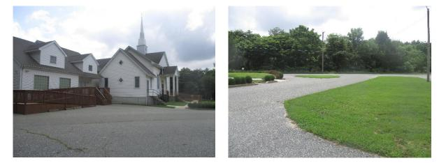
Stormwater currently drains from the property to the roadway. A bioswale placed on the east side of the island in the middle of the parking lot can capture, treat, and infiltrate roof runoff and stormwater runoff from a good portion of the parking lot. A preliminary soil assessment suggests that the soils have suitable drainage characteristics for green infrastructure.
