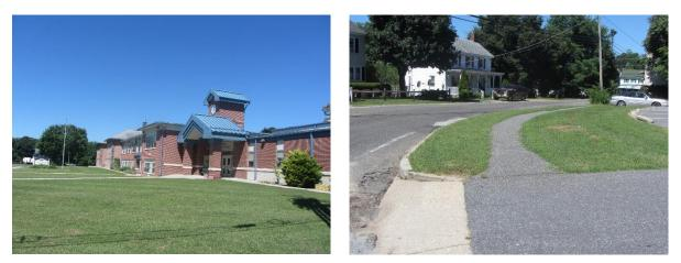
Stormwater is currently directed to existing catch basins and the roadway. Parking spots on the west side of the building can be replaced with porous asphalt to capture and infiltrate stormwater. Rain gardens adjacent to the building and the west parking lot can capture, treat, and infiltrate stormwater and roof runoff. A preliminary soil assessment suggests that the soils have suitable drainage characteristics for green infrastructure.
