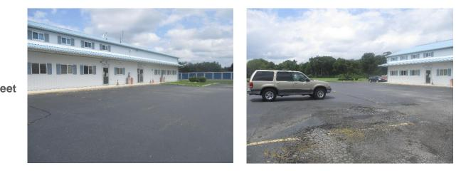
Stormwater is currently directed to existing catch basins. The main parking lot is in poor shape, and parking spots can be replaced with porous asphalt to capture and infiltrate stormwater runoff. A preliminary soil assessment suggests that the soils have suitable drainage characteristics for green infrastructure.
